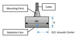
Transmitting Voltage Response (TVR) and Free-field Voltage Sensitivity (FFVS):
