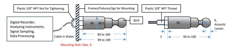
3. Thru-hole Mounting (Inch Thread) with Single O-ring Sealing THM-7/16" (7/16"-20x22 UNF-2A).
