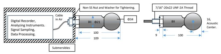
4. Bolt-Fastening Mounting BFM-7/16" (7/16"-20x22 UNF-2A).
