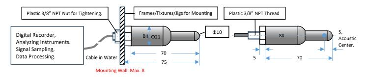
3. Thru-hole Mounting (Inch Thread) with Single O-ring Sealing THM-7/16" (7/16"-20x22 UNF-2A).
