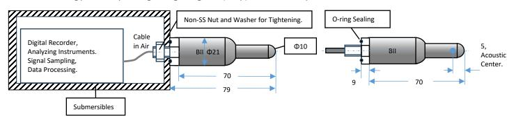
4. Bolt-Fastening Mounting BFM-7/16" (7/16"-20x22 UNF-2A).
