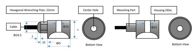
Cylindrical Sector Aperture (Dimensional Unit: mm): 1. Cable goes out of the device from the rear.
