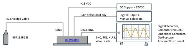
How do I use Gain Selection wires of a standalone PGA in field?
