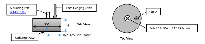
2. Bolt-Fastening Mounting BFM-7/16" (7/16"-20x22 UNF-2A) for Small Transducer, or BFM-5/8" (5/8"-18x22 UNF) for Large Transducer.
