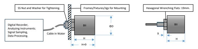
3. Thru-hole Mounting with Single O-ring Sealing THM-7/16" (7/16"-20x22 UNF-2A) for Small Transducer, or THM-5/8" (5/8"-18x22 UNF) for Large Transducer.
